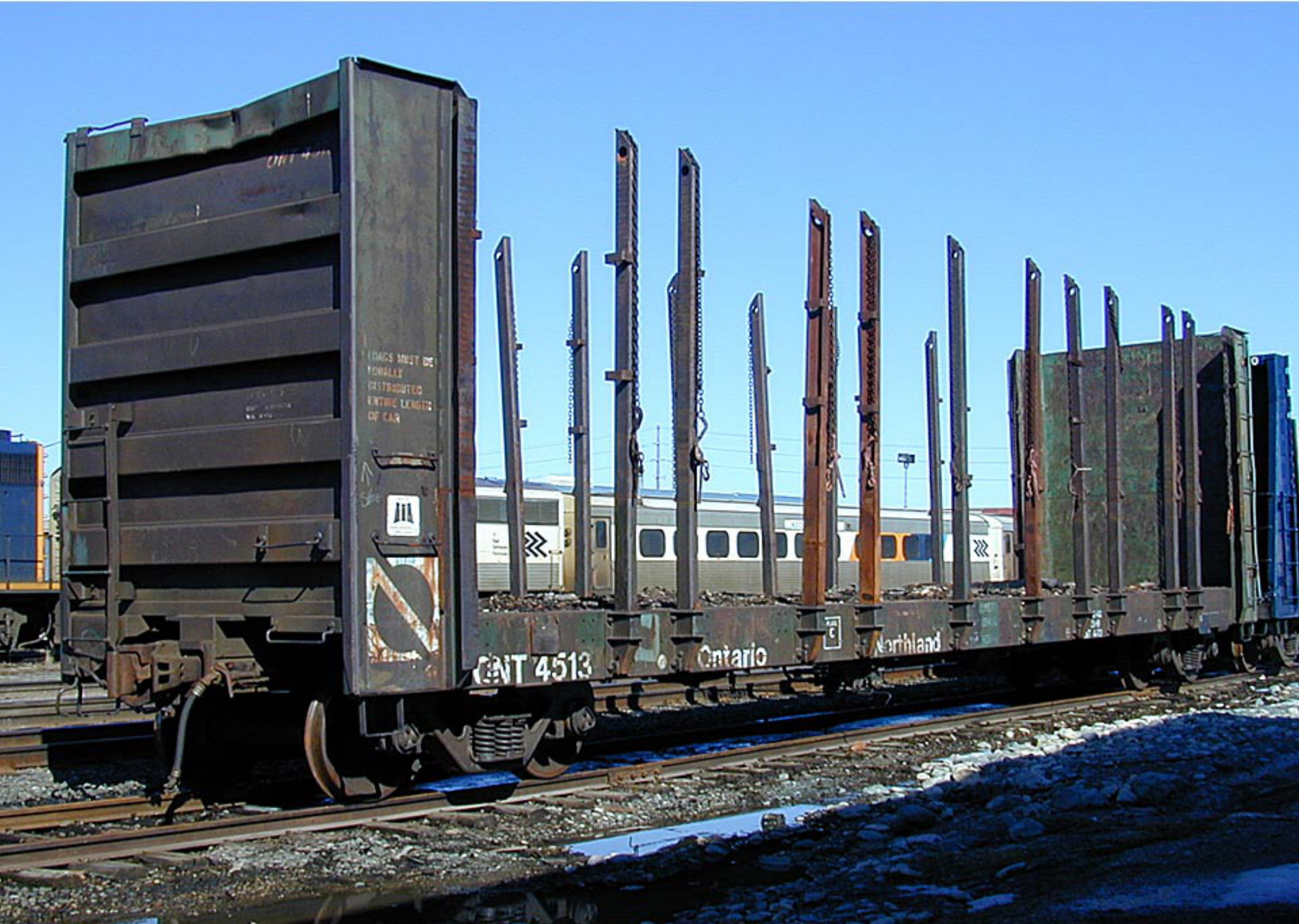
Gareth Bayer's North American RR Images I Ontario Northland bulkhead flat (pulpwood) No. ONT 4513 @ Cochrane Yard, ON., 13th April 2002 © 2004 Gareth Bayer <gareth.bayer@btopenworld.com>
